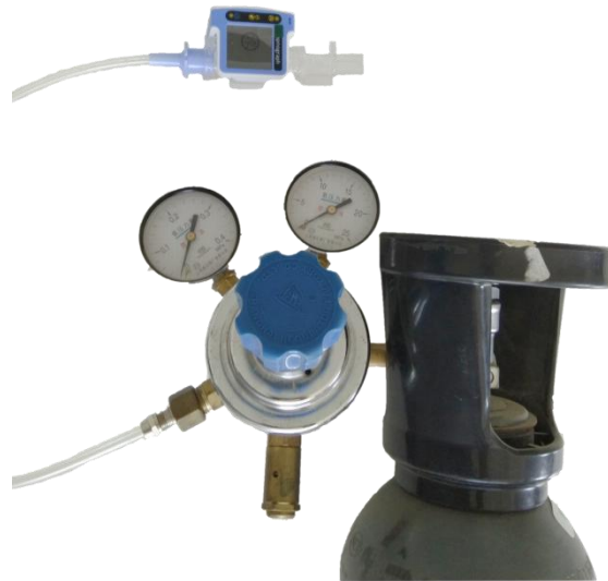
Figure 10. Gas span check connection
