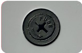
The fuse is located on the bottom of the device
